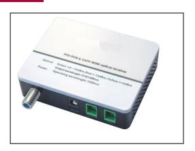
FTTH broadband access is the ultimate devolopment goal, ON600WD is the target terminal product fort his. It adopts technology of high isolation WDM in order to separate CATV and ONU signal. Furthermore, it also adopts low optical power receiving and RF-AGC control technique, which could achieve the requirement of  $\leq$ -10dBm CATV receiving for FTTH. It supports RF outputs constantly.
